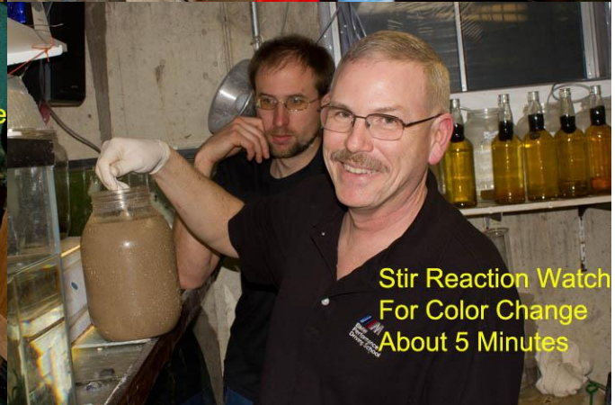
Add ICE COLD Bleach and a DASH of 50% Sodium Hydroxide
